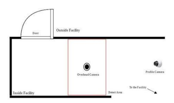
Figure 3: Position of overhead camera with narrow passageway
